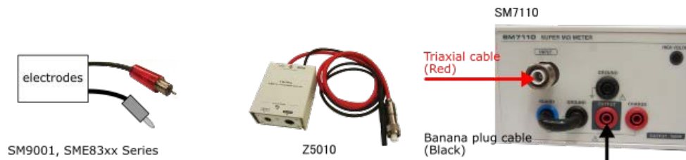
Figure 7-7. How to connect electrodes to the SM7110
