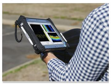
Combined with a Tektronix USB spectrum analyzer, the Panasonic FZ-G1 transforms your view of the spectrum in the field. It provides the largest screen of any portable solution and weighs but a fraction of a traditional portable spectrum analyzer in your
