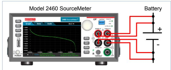
Figure 12. Results of discharging battery shown on graphical display of Model 2460 SourceMeter SMU instrument
