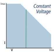
Constant voltage mode is used for load testing of constant current power supplies. The unit operates as a high power shunt regulator.
