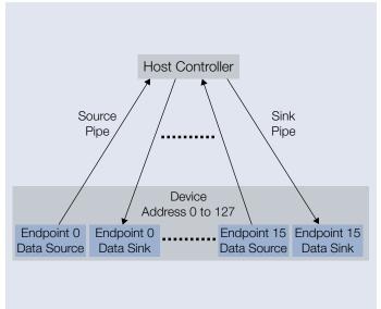
A USB network includes one host controller and from 1 to 127 devices. USB is a tiered-star topology with optional hubs to expand the bus. The host is the only master and it controls all bus traffic. The host initiates all device communications and devices do not have the capability to interrupt the host.
