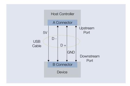
A twisted differential pair Data+ (D+ green wire) and Data- (D- white wire) wires are used for bidirectional communications using half-duplex differential signaling controlled by the host. On an oscilloscope the individual signals can be captured using passive or active analog probes, as well as digital logic probes.
