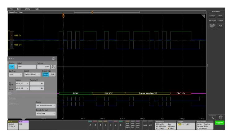
This case shows full-speed USB 2.0 traffic between a PC and a USB drive. A logic probe connected to a FlexChannel® input is used to capture the signals. Although the oscilloscope can acquire and decode lower-speed USB bus signals using single-ended probing, the signal fidelity and noise immunity is improved by using differential probing, and is a necessity for high-speed USB signals.
