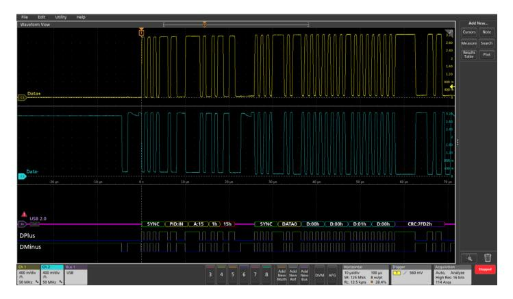
When the mouse is moved, it responds to the host request with a series of data bytes indicating the change of position.
