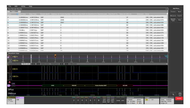
For firmware engineers, the Results Table format may be more useful. This time-stamped display of bus activity can be easily compared to the software listings, and provides easy calculation of the execution speed.
