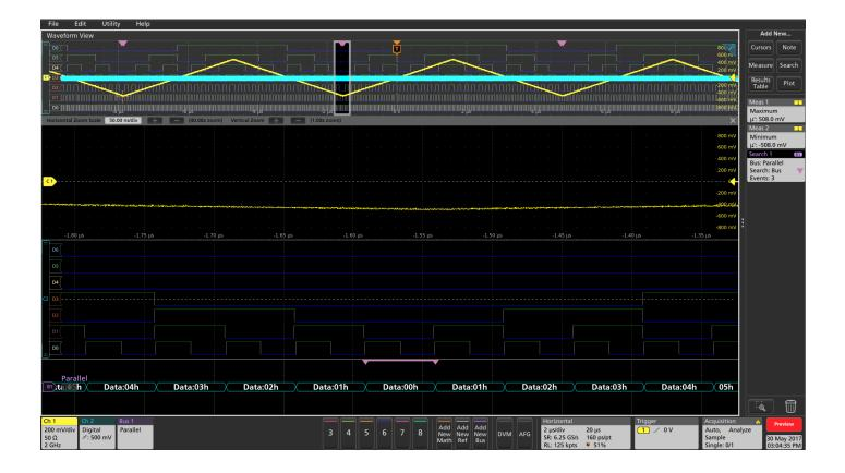
Configuring Wave Inspector to search for 00 hex values yields the expected results as well. There are now three 00 hex values found in the waveform record, one for each test ramp valley. The signal conditioning circuit adjustments resolved the issue, and the test ramp now correctly exercises each available digitizing level in the 6-bit Analog to Digital Converter.
