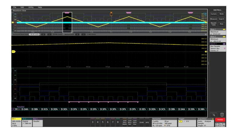
Reconfiguring the Wave Inspector Search and Mark for the maximum ADC output value of 3F yields 21 results. This should throw up warning flags, as there should only be three 3F values, one for each test signal peak. Looking at the zoom overview, the marks for the 3F values are grouped in three bunches over each test ramp peak. The zoom view over the decoded parallel bus values shows the expected progression of values 3A, 3B, 3C, 3D, 3E, up to 3F where instead of a single value there are seven.
