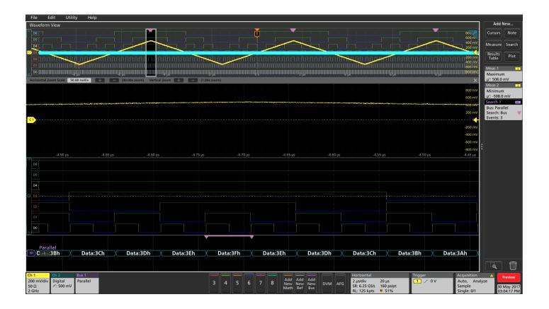
After adjusting the gain and offset of the signal conditioning circuit, the ADC input waveform maximum and minimum is now a symmetrical 508 mV and -508 mV respectively. There is now a single 3F hex value at each test ramp peak as expected. The maximum input of the ADC is now correctly sampled.
