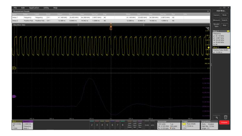
Now that we know that the frequency occasionally decreases, we can use pulse width triggering to capture abnormally wide pulses and capture the errors. In this example, the scope is set to trigger on a pulse width greater than 14 ns, which is more than the nominal 12.5 ns. The frequency trend at the bottom of the display shows graphically the frequency excursion above and below the 40 MHz ideal.
