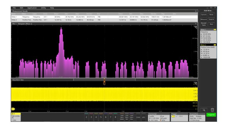
Now that we know these variations are there, we can plot the frequency measurements on a histogram with a logarithmic Y-axis to better understand the variations. (Using the logarithmic scale lets us see more detail at the low end of the scale.)
