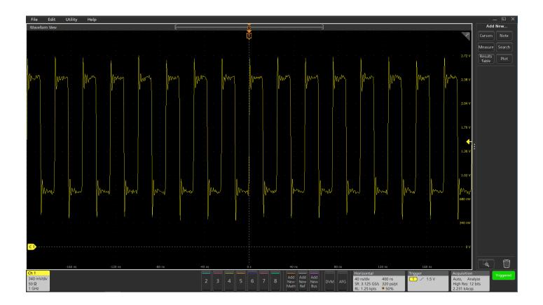
This display shows a 40 MHz clock signal captured with 12-bit vertical resolution on a 1 GHz bandwidth 5 Series MSO. To assure adequate signal fidelity, a 1 GHz differential probe was attached to the test points near the clock driver. Since the bandwidth of the measurement system is about 25 times the clock frequency, measurement errors due to bandwidth are minimal.
