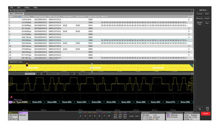
Adding the Results Table view of the decoded information provides a timestamped display of the bus activity that can be easily compared to the software listings. Tapping a line in the Results Table automatically zooms in on the corresponding bus signals and resulting decoded bus waveform, shown in the lower section of the display.
