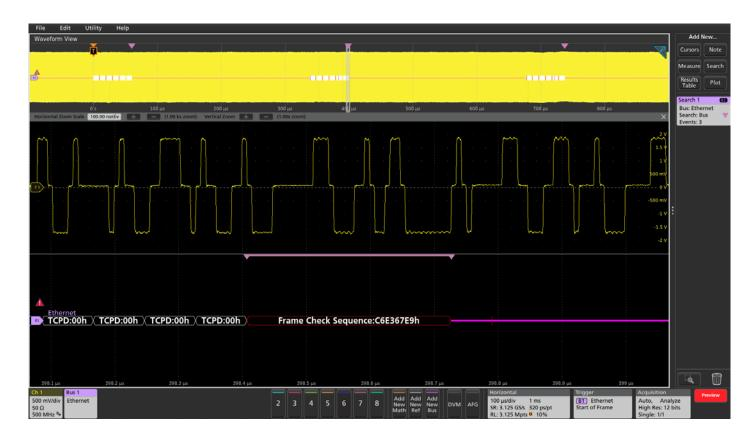
The decoded bus display above shows that three bursts of bus activity were captured. To find specific values in the activity, you can use Wave Inspector automatic search to mark each specified evet. In this example, the automated bus search is configured to find all Frame Check Sequence errors and it shows 3 events, at the end of each burst of bus activity.
