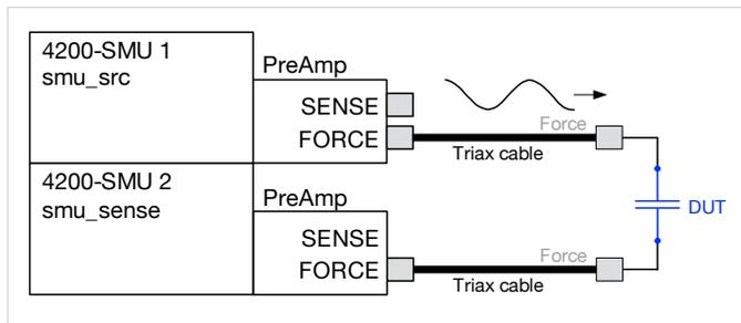
Figure 7. VLF C-V connections for the capacitor. If the test device is on wafer, see the MOSCap diagram (**Figure 2**) for connections.
