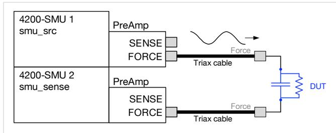
Figure 13. Connection diagram for parallel RC test device.
